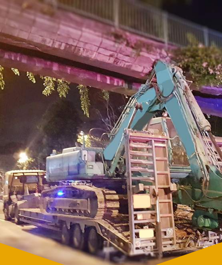
Inadequately retracted crane ❌
