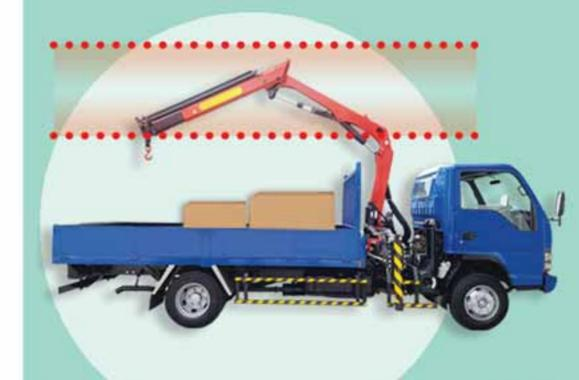
Remember to retract the crane adequately before driving!
