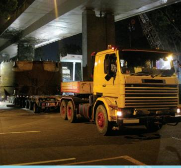
Heavy vehicles which are used to carry large and heavy cargo tend to slow down traffic. They may also affect road structures due to their large dimension and heavy weight. To ensure the safety of road users, movement of such vehicles has to be controlled.
